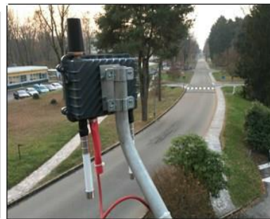
ITS-G5 RSU deployed in the JRC Ispra campus
