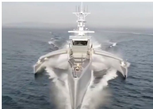
2017–2018/ Trimaran–Drone “Sea Hunter” DARPA US/Navy . 1 st Autonomous–Unmanned Vessel (MDUSV)
