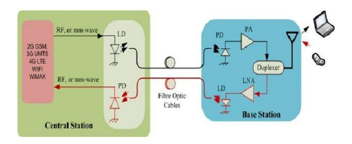
Integration of wireless and fibre optic communication technologies, and modulating wireless signals over optical carrier for transporting over fibre optic cable.
