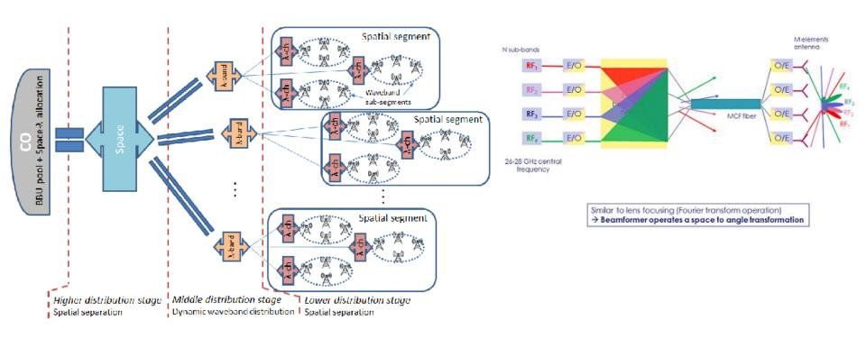
Optical Beamforming: carries the RF signals in MCF to the antenna arrays
