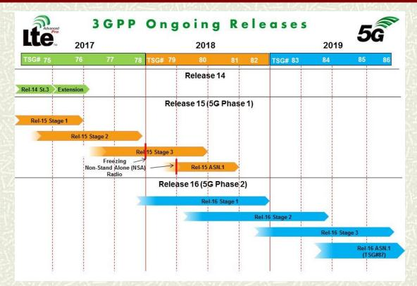
End of 2017 the non-standalone 5G access is completed. The new 5G access scheme is using dual connectivity with LTE as the master eNB and does not need a specification of a full 5G radio resource control. The standalone 5G radio access network that will be connected to the 5G core is be completed in Release 15 (mid of 2018).
