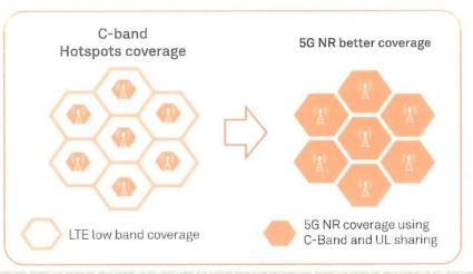
An important feature of the **3GPP Release 15** standard resides in the ability for LTE and 5G NR to co-exist and share the same low frequency bands without having to fully free those bands from LTE use. In the initial stage of 5G deployment, the new bands likely to be made available for 5G are higher in frequency (e.g. C-band) and support less sub-frames for uplink than most existing 2G/3G/4G bands. Such bands will therefore have more uplink coverage limitations compared to existing bands.
