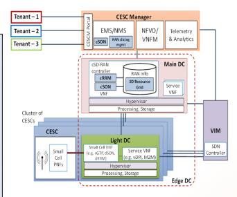
In the CESC, rather than providing multiple S1 (or Iu-h interface) connections from the physical SC to different operators' EPC network elements such as Mobility Management Entity (MME) and SGW, such fan-out is done at the Light DC. The CESC is further the termination of multiple S1 interfaces connecting the CESC to multiple MME/SGW entities as in S1-Flex.
