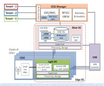
**The CESCM also encompasses a telemetry and analytics module that captures and analyses relevant indicators of the network operation.** This will provide the CESCM with accurate knowledge models that characterise the behaviour of the network and its users in relation to the utilisation of both cloud and radio resources. **This will facilitate the realisation of effective optimisation approaches** based on, for example, machine learning (ML)
