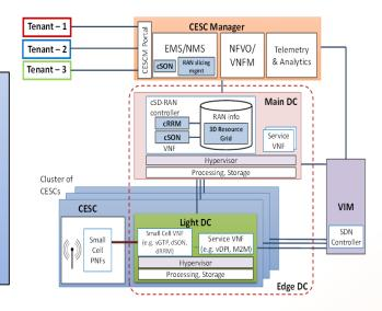
The role of VIM is essential for the deployment of NFV services and to form and provide a layer of NFV resources to be made available to the CESCM functions.
