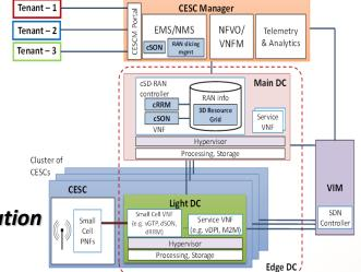
Edge cloud computing and networking are realised through the sharing of computation, storage and network resources of those micro-servers present in each CESC and these form the Light DC, for implementing different features/capabilities of the SC. Therefore, the CESCs becomes a "neutral host" for network operators or virtual network operators that want to "share" IT and network resources at the edge of the mobile network.
